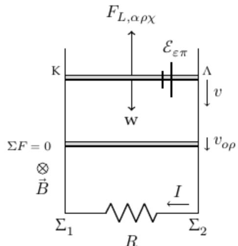
$$\frac{dE_{\text{MHX}}}{dt} = \frac{dK}{dt} + \frac{dU}{dt} = (\Sigma F \cdot v) + (-mgv) = -F_L v = -160 \text{ J/s}$$
